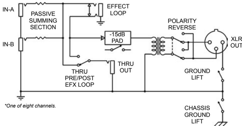
As previously mentioned, the ‘engine’ inside the ProD8 is the Radial transformer. This ‘hi-Z to lo-Z’ device is designed to convert the impedance and balance the signal so that it matches the level of a typical microphone. This way, the keyboards connected to the ProD8 can be ‘managed’ just like microphones and used with mic splitters as well as the mic inputs on the mixing console. A polarity reverse switch toggles pins 2 and 3 to allow older pre-AES standard gear to be connected in phase.
