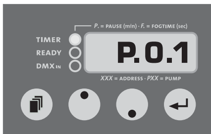
Adjusting of the wait time in minutes (0.1-99)
