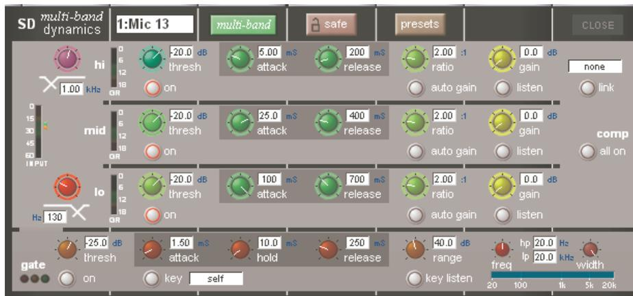
Up to 8 Channels can have their Dynamics (Compressor) modules switched into Multi-band mode
