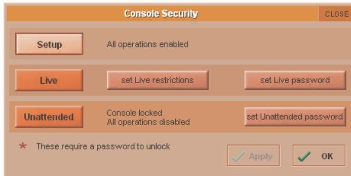
User passwords can be defined for the Live and Unattended modes. To set a password, press the Set Password button. Enter the old password, then enter the new password.
