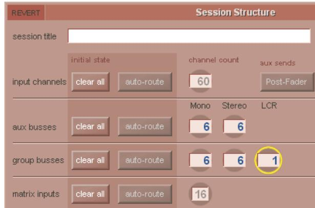
If an LCR Buss exists within the session, it is automatically assumed to be the Master buss, and the dedicated Master fader is automatically assigned to the LCR buss.
