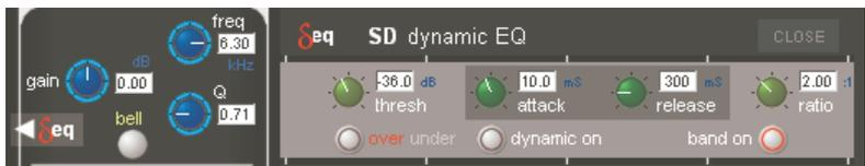
To place the dynamic module into Over mode, ensure that the Over indication below the threshold control is not illuminated.
