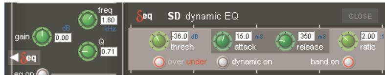
To place the dynamic module into Under mode, ensure that the Over indication below the threshold control is illuminated.
