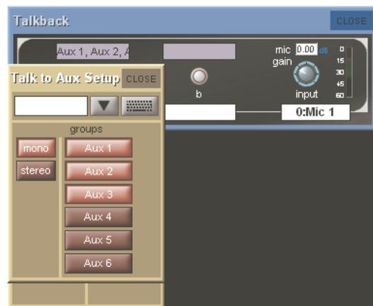
On the Aux Output channels hold one of the Assign buttons next to the rows of assignable controls and then touch the talk section on screen. This will assign the selected rotary control and switch to be **Talk Level** and **Talk On/Off**.
