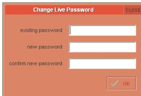
**NOTE:** If you should forget your password, call your Distributor to obtain a reset password. Entering the master override password will delete all of the user-set passwords, allowing new passwords to be set.
